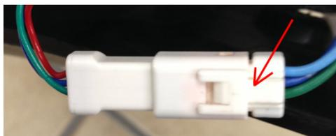
4. Connect the pins just loosened with the pins of the bikespeed cable set.
