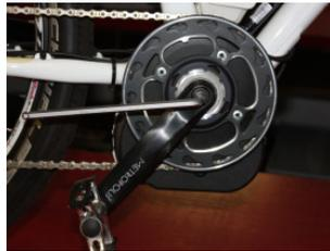
2. Dismount the treadle with a suitable crank puller (e.g. picture: Lifu, used for most bicycles with a Bosch-engine)
