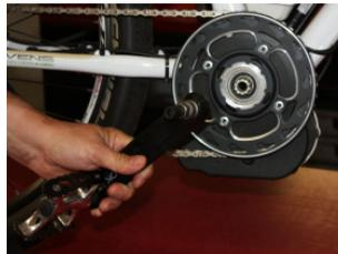
3. Remove the screw nut of the chain ring (Spider).
