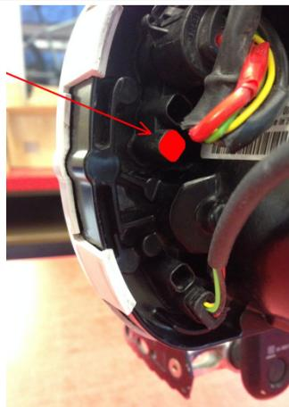
The removed plug is two-pole and grey.
