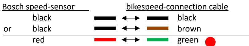
The screw terminal for the green conductor of the bikespeed-cable set is additionally marked with a red point.
