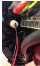
The plug has to be inserted as far as it will go. The silicon seal may no longer be visible. Upon delivery we apply some Vaseline onto the seals for lubrication. If there is not enough lubrication, you may renew it. Please advance with care when you insert the plug. Do not use force!
