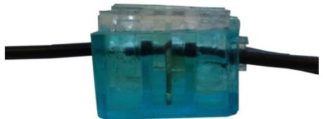
Use a pair of combination pliers for the final squeeze and press so long that the visible part of the terminal clicks flush into place in the blue part.
