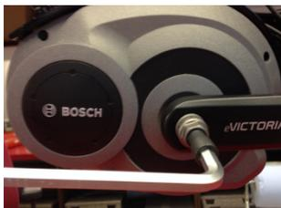
3. Remove the three screws of the gravel deflector. (tool: Torx T20)
