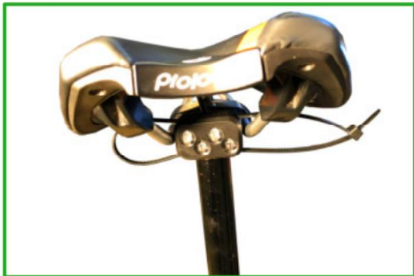
Then tighten the cable tie and cut off the protruding end (for example with a side cutter)
