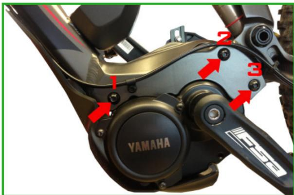
**2. It is possible that your motor is attached to more screws of further covers. These must be removed as well. (see example):**
