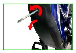
**2.** Below the cover you will find the connector to the battery. Disconnect it by turning the bayonet lock counterclockwise and then pulling the plug downward.
