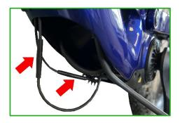
**10.** Stow the bikespeed-RS in the frame. You will find sufficient space for this in the direction shown in the photo.
