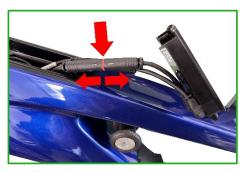
8. The two longer cables on the bikespeed-RS must be routed through the frame down to the motor. You can see the cable routing by the arrows. A cable puller is required for this step. This is pushed into the frame best from below the motor. This is possible without removing the motor.
