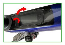
Disconnect the connector from the display to the motor. This can be recognized by the red ring. Plug these connectors to the counterparts on the bikespeed-RS.
