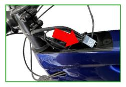
**11.** Mount the display by snapping it back into the frame at the bottom side, then fold it inside and secure it with the screw.
