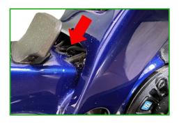
The connector to the speed sensor is needed at the front of the motor. (see first photo step 5)
