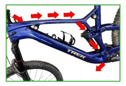
Tie the two connectors of the bikespeed-RS to the cable puller and carefully pull it through the frame to the motor.
