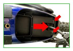
**5.** Locate the connector to the speed sensor. This is black, round and has a diameter of approx. 5mm.
