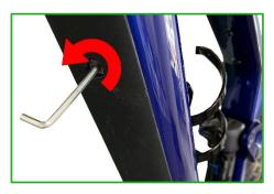
Pull the battery downwards out of the frame. Then loosen the two screws of the cable cover behind the battery with a Torx T15. Pull the cover out downwards.
