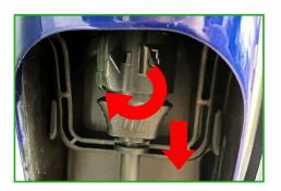
3. Loosen the upper fastening screw of the battery. (also with a size 4 Allen key)
