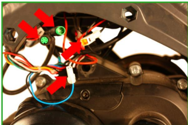
5. Connect the 4 connectors of the bikespeed-RS with the newly released connectors. The tuning is simply interposed.
