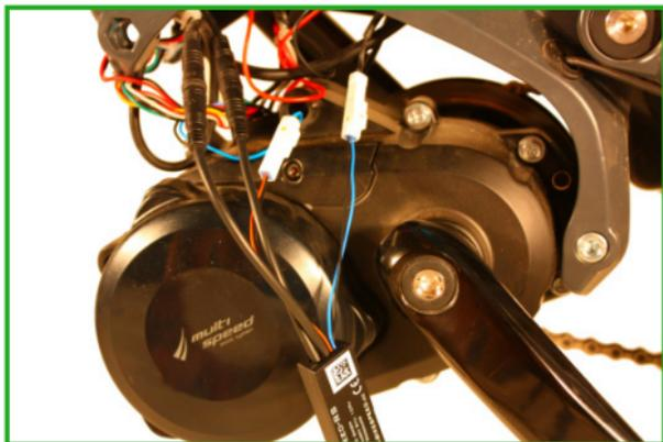
6. Stow the bikespeed-RS as well as all connectors and cables in the frame tube.
