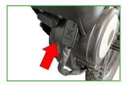
Replace the lower gravel deflector and secure it with the four screws. Be sure to use the correct front and rear screws. (See note from step 4)
