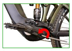
4. Loosen the four screws of the lower gravel deflector with a size 2.5 Allen key and remove it. Note: Different screws are used at the front and rear. Please note the position for later correct mounting.
