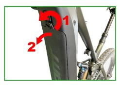
Loosen the battery mounting screw with a Torx T25 or your battery key. Note: This is an endless screw that cannot be removed.
