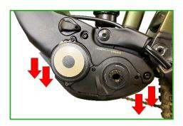
Disconnect the two connectors for the display (6-pin, labeled "Info") and the speed sensor (3-pin, labeled "SS"). The connectors are held in place with a latching tab. You simply release this with a slight pressure with your fingernail or a narrow screwdriver.
