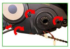
Connect the two connectors of the bikespeed-RS to the slots on the motor where you disconnected the original connectors in step 5.
