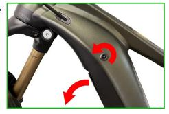
Loosen the screw of the left pedal crank with a size 8 Allen key. The screw also functions as a crank puller. Turn it until you can remove the crank.
