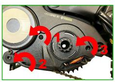
Connect the two connectors disconnected in step 5 to the corresponding counterparts on your bikespeed-RS and place the connectors at the locations marked with arrows:
