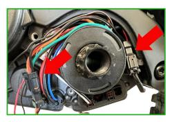
Replace the side cover. Guide the two remaining connectors of the bikespeed-RS out of the opening at the bottom right and guide the cable to the bikespeed-RS out of the cover on the left. (See arrow) Then fasten the cover again with the three screws. Make sure that you do not squeeze cables!
