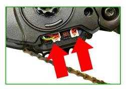
**10.** Stow the bikespeed-RS in the position shown in the frame.
